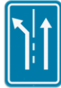
Figure 27 This F13 information traffic board shows arrows on the roadway to help you choose the right lane.
